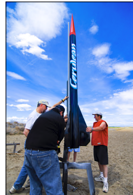
Neil Anderson's "Cerulean" being prepared to launch on a 98mm "N" 'Green Gorilla' motor.
